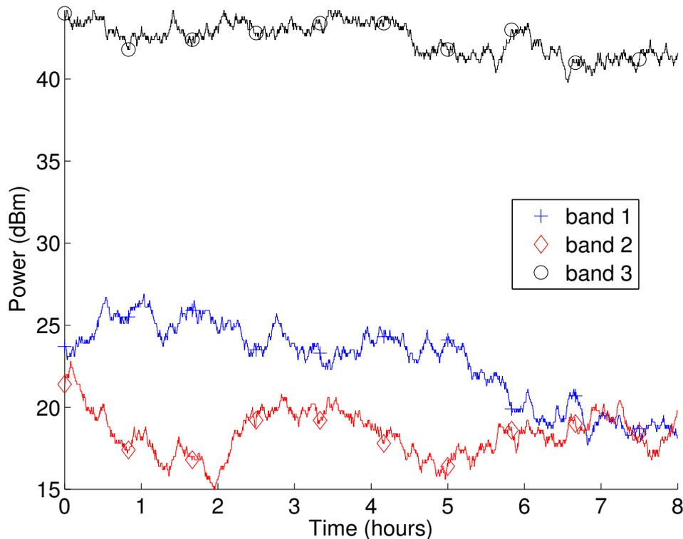
Fig. 3. Powers on different sub-bands transmitted by BS 2 as a function of time for FFR
