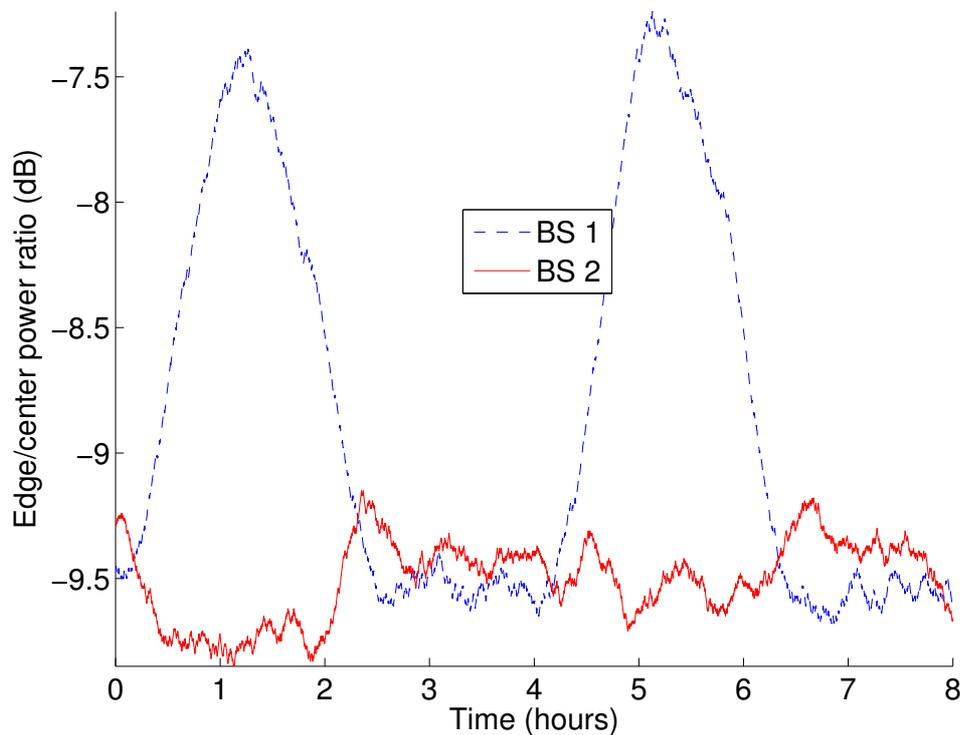
Fig. 5. Edge/center power ratio for BS 1 and 2 as a function of time for SFR
